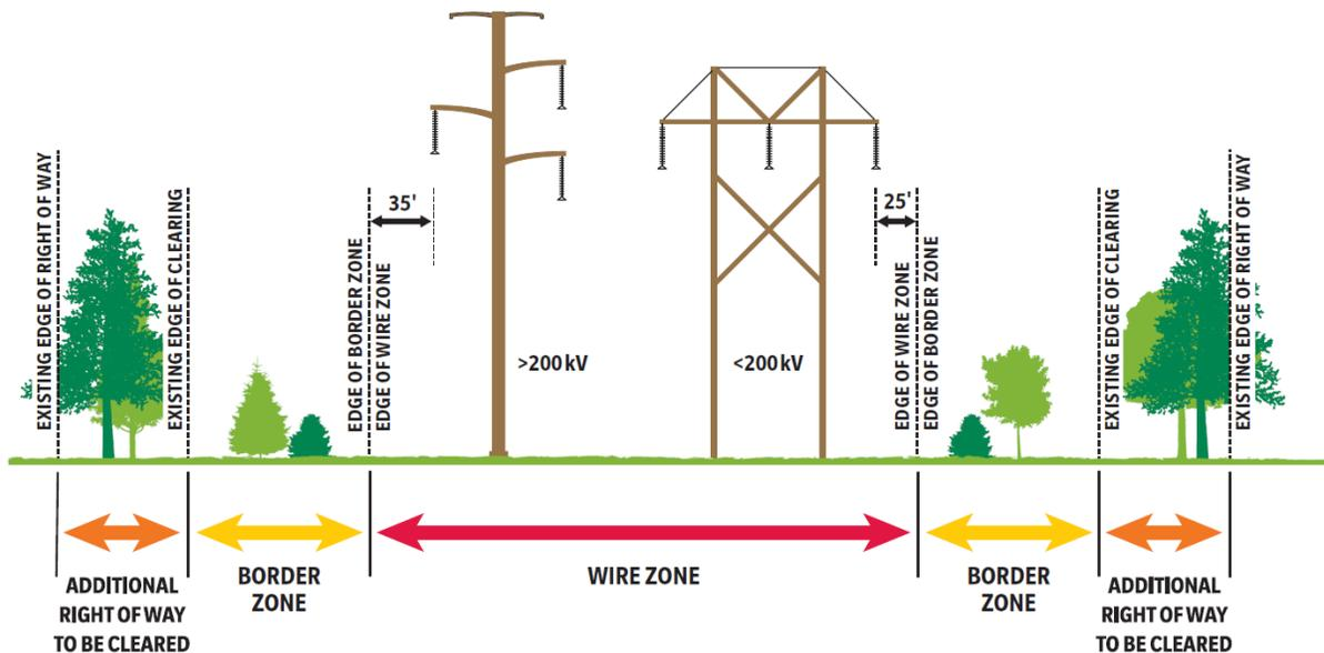
*This diagram is for illustrative purposes. Your neighborhood may have a different configuration of transmission structures. Distances shown are the minimum clearances from the conductors and may be greater based on line construction.*
